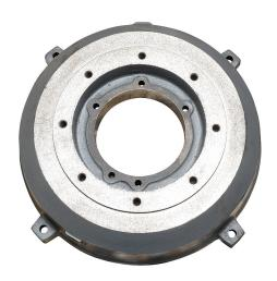
IronHorse C-flange, replacement. For use with 405T frame IronHorse premium efficiency MTCP2 series motors. Mounting hardware included. Replaces drive end bell, field install. Not compatible with MTC or MTCP series motors.
