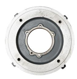
IronHorse C-flange, replacement. For use with 324T and 326T frame IronHorse premium efficiency MTCP2 series motors. Mounting hardware included. Replaces drive end bell, field install. Not compatible with MTC or MTCP series motors.
