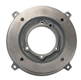
IronHorse C-flange, replacement. For use with 284T and 286T frame IronHorse premium efficiency MTCP2 series motors. Mounting hardware included. Replaces drive end bell, field install. Not compatible with MTC or MTCP series motors.
