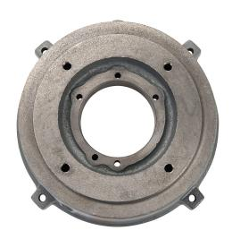
IronHorse C-flange, replacement. For use with 254T and 256T frame IronHorse premium efficiency MTCP2 series motors. Mounting hardware included. Replaces drive end bell, field install. Not compatible with MTC or MTCP series motors.
