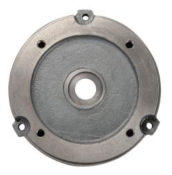
IronHorse C-flange, replacement. For use with 182T and 184T frame IronHorse premium efficiency MTCP2 series motors. Mounting hardware included. Replaces drive end bell, field install. Not compatible with MTC or MTCP series motors.
