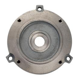
IronHorse C-flange, replacement. For use with 143T and 145T frame IronHorse premium efficiency MTCP2 series motors. Mounting hardware included. Replaces drive end bell, field install. Not compatible with MTC or MTCP series motors.
