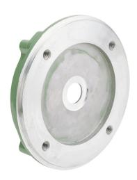
IronHorse C-flange, replacement. For use with 182T and 184T frame IronHorse MTF2 series 1-phase motors. Mounting hardware included. Replaces drive end bell, field install. Not compatible with MTF series motors.
