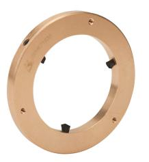
IronHorse current diverter ring, for use with 284T and 286T frame drill and tap motors. MTDP series motors are drilled and tapped for mounting current diverter rings, others will require drilling and tapping to mount.
