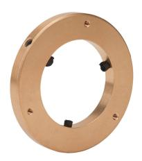
IronHorse current diverter ring, for use with 213T and 215T frame drill and tap motors. MTDP series motors are drilled and tapped for mounting current diverter rings, others will require drilling and tapping to mount.
