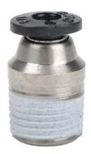
NITRA pneumatic push-to-connect fitting, male, round straight, nickel-plated brass body, nickel-plated brass threads, 1/8in tube to 1/8in NPT connection(s). Package of 5.
