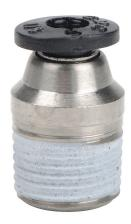
NITRA pneumatic push-to-connect fitting, round straight, nickel-plated brass body, nickel-plated brass threads, thread sealant, (1) 1/8in male NPT to (1) 1/8in push-to-connect. Package of 5.
