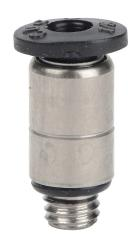
NITRA pneumatic push-to-connect fitting, round straight, nickel-plated brass body, nickel-plated brass threads, thread sealant, (1) #10-32 male UNF to (1) 1/8in push-to-connect. Package of 5.
