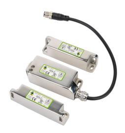
IDEM standalone safety switch set, dual non-contact coded magnetic, automatic restart, (2) N.C. safety output(s), 316 stainless steel housing, 38mm x 95mm body, 8-pin M12 quick-disconnect, 9.8in/250mm cable length.
