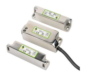
IDEM standalone safety switch set, dual non-contact coded magnetic, manual or automatic restart, (2) N.C. safety output(s), (1) status monitoring output(s), 316 stainless steel housing, 38mm x 95mm body, pigtail, 32.8ft/10m cable length.
