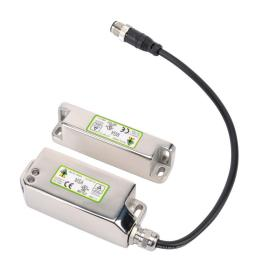
IDEM standalone safety switch set, non-contact coded magnetic, manual restart, (2) N.C. safety output(s), 316 stainless steel housing, 38mm x 95mm body, 8-pin M12 quick-disconnect, 9.8in/250mm cable length.
