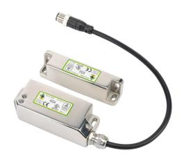
IDEM standalone safety switch set, non-contact coded magnetic, automatic restart, (2) N.C. safety output(s), 316 stainless steel housing, 38mm x 95mm body, 8-pin M12 quick-disconnect, 9.8in/250mm cable length.
