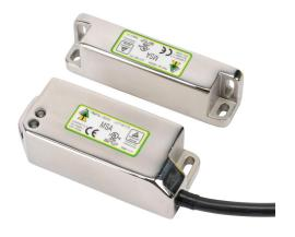
IDEM standalone safety switch set, non-contact coded magnetic, manual or automatic restart, (2) N.C. safety output(s), (1) status monitoring output(s), 316 stainless steel housing, 38mm x 95mm body, pigtail, 32.8ft/10m cable length.
