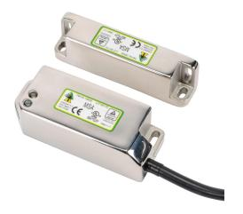
IDEM standalone safety switch set, non-contact coded magnetic, manual or automatic restart, (2) N.C. safety output(s), (1) status monitoring output(s), 316 stainless steel housing, 38mm x 95mm body, pigtail, 16.4ft/5m cable length.
