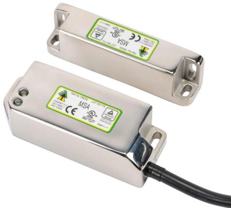
IDEM standalone safety switch set, non-contact coded magnetic, manual or automatic restart, (2) N.C. safety output(s), (1) status monitoring output(s), 316 stainless steel housing, 38mm x 95mm body, pigtail, 16.4ft/5m cable length.
