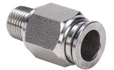
NITRA pneumatic push-to-connect fitting, male, straight, 316 stainless steel body, 316 stainless steel threads, 5/16in (8mm) tube to R1/8 BSPT connection(s).
