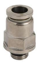
NITRA pneumatic push-to-connect fitting, male, straight, nickel-plated brass body, nickel-plated brass threads, thread sealant, 5/16in (8mm) push-to-connect to G1/8 BSPP. Package of 5.
