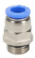
NITRA pneumatic push-to-connect fitting, straight, nickel-plated brass body, nickel-plated brass threads, thread sealant, (1) G1/4 male BSPP to (1) 5/16in (8mm) push-to-connect. Package of 5.
