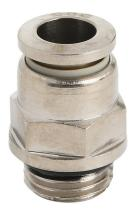
NITRA pneumatic push-to-connect fitting, straight, nickel-plated brass body, nickel-plated brass threads, thread sealant, (1) G1/4 male BSPP to (1) 5/16in (8mm) push-to-connect. Package of 5.
