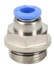
NITRA pneumatic push-to-connect fitting, straight, nickel-plated brass body, nickel-plated brass threads, thread sealant, (1) G3/8 male BSPP to (1) 6mm push-to-connect. Package of 5.
