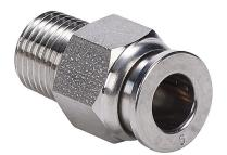
NITRA pneumatic push-to-connect fitting, straight, 316 stainless steel body, 316 stainless steel threads, (1) R1/8 male BSPT to (1) 6mm push-to-connect.
