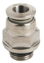
NITRA pneumatic push-to-connect fitting, straight, nickel-plated brass body, nickel-plated brass threads, thread sealant, (1) G1/8 male BSPP to (1) 6mm push-to-connect. Package of 5.
