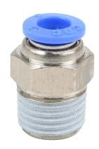
NITRA pneumatic push-to-connect fitting, straight, nickel-plated brass body, nickel-plated brass threads, thread sealant, (1) R1/4 male BSPT to (1) 6mm push-to-connect. Package of 5.
