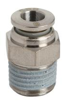
NITRA pneumatic push-to-connect fitting, straight, nickel-plated brass body, nickel-plated brass threads, thread sealant, (1) R1/4 male BSPT to (1) 6mm push-to-connect. Package of 5.
