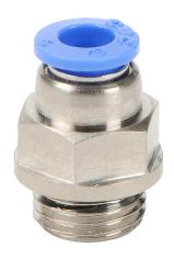
NITRA pneumatic push-to-connect fitting, straight, nickel-plated brass body, nickel-plated brass threads, thread sealant, (1) G1/4 male BSPP to (1) 6mm push-to-connect. Package of 5.
