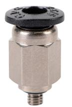
NITRA pneumatic push-to-connect fitting, straight, nickel-plated brass body, nickel-plated brass threads, thread sealant, (1) M3 x 0.5 male ISO to (1) 5/32in (4mm) push-to-connect. Package of 5.
