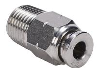
NITRA pneumatic push-to-connect fitting, straight, 316 stainless steel body, 316 stainless steel threads, (1) 1/8in male NPT to (1) 5/32in (4mm) push-to-connect.
