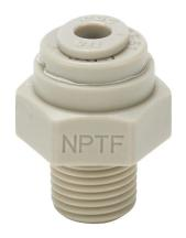
HydroMode potable water push-to-connect fitting, male, straight, acetal body, acetal threads, (1) 5/32in tube to (1) 1/8in male NPT connection(s), NSF/ANSI 61. Package of 5.
