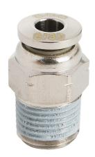
NITRA pneumatic push-to-connect fitting, straight, nickel-plated brass body, nickel-plated brass threads, thread sealant, (1) 1/8in male NPT to (1) 5/32in (4mm) push-to-connect. Package of 5.
