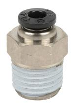
NITRA pneumatic push-to-connect fitting, straight, nickel-plated brass body, nickel-plated brass threads, thread sealant, (1) 1/4in male NPT to (1) 5/32in (4mm) push-to-connect. Package of 5.
