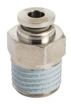
NITRA pneumatic push-to-connect fitting, straight, nickel-plated brass body, nickel-plated brass threads, thread sealant, (1) 1/4in male NPT to (1) 5/32in (4mm) push-to-connect. Package of 5.
