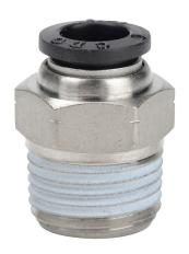
NITRA pneumatic push-to-connect fitting, straight, nickel-plated brass body, nickel-plated brass threads, thread sealant, (1) 3/8in male NPT to (1) 5/16in (8mm) push-to-connect. Package of 5.
