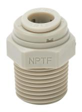
HydroMode potable water push-to-connect fitting, male, straight, acetal body, acetal threads, (1) 5/16in tube to (1) 3/8in male NPT connection(s), NSF/ANSI 61. Package of 5.
