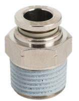
NITRA pneumatic push-to-connect fitting, male, straight, nickelplated brass body, nickel-plated brass threads, thread sealant, 5/16in (8mm) push-to-connect to 3/8in NPT. Package of 5.
