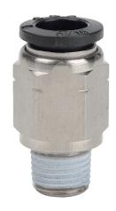
NITRA pneumatic push-to-connect fitting, straight, nickel-plated brass body, nickel-plated brass threads, thread sealant, (1) 1/8in male NPT to (1) 5/16in (8mm) push-to-connect. Package of 5.
