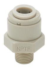
HydroMode potable water push-to-connect fitting, male, straight, acetal body, acetal threads, (1) 5/16in tube to (1) 1/8in male NPT connection(s), NSF/ANSI 61. Package of 5.
