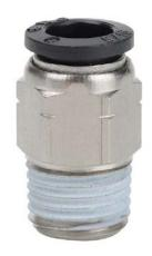
NITRA pneumatic push-to-connect fitting, male, straight, nickel-plated brass body, nickel-plated brass threads, 5/16in (8mm) tube to 1/4in NPT connection(s). Package of 5.
