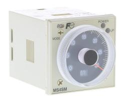
Fuji Electric multi-mode relay timer, 0.05 seconds to 60 hours selectable timing range, 24 VAC/VDC operating voltage, 5A contact rating, (1) DPDT timed relay output(s), socket mount, 11-pin. Requires Fuji Electric TP411X or TP411SBA timer socket.
