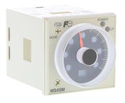
Fuji Electric multi-mode relay timer, 0.05 seconds to 60 hours selectable timing range, 100-240 VAC operating voltage, 5A contact rating, (1) DPDT timed relay output(s), socket mount, 11-pin. Requires Fuji Electric TP411X or TP411SBA timer socket.
