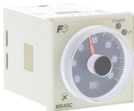
Fuji Electric on-delay relay timer, 0.05 seconds to 60 hours selectable timing range, 24 VAC/VDC operating voltage, 5A contact rating, (1) SPDT timed relay and (1) SPDT instant relay output(s), socket mount, 8-pin. Requires Fuji Electric TP48X or TP48SB timer socket.
