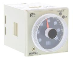
Fuji Electric on-delay relay timer, 0.05 seconds to 60 hours selectable timing range, 100-240 VAC operating voltage, 5A contact rating, (1) SPDT timed relay and (1) SPDT instant relay output(s), socket mount, 8-pin. Requires Fuji Electric TP48X or TP48SB timer socket.
