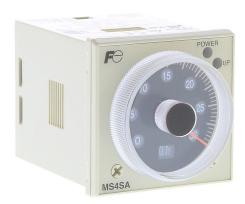
Fuji Electric on-delay relay timer, 0.05 seconds to 60 hours selectable timing range, 24 VAC/VDC operating voltage, 5A contact rating, (1) DPDT timed relay output(s), socket mount, 8-pin. Requires Fuji Electric TP48X or TP48SB timer socket.
