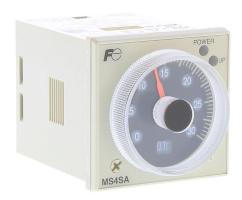
Fuji Electric on-delay relay timer, 0.05 seconds to 60 hours selectable timing range, 100-240 VAC operating voltage, 5A contact rating, (1) DPDT timed relay output(s), socket mount, 8-pin. Requires Fuji Electric TP48X or TP48SB timer socket.
