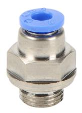
NITRA pneumatic push-to-connect fitting, straight, nickel-plated brass body, nickel-plated brass threads, thread sealant, (1) G1/8 male BSPP to (1) 5/32in (4mm) push-to-connect. Package of 5.
