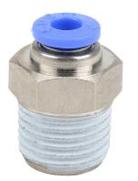
NITRA pneumatic push-to-connect fitting, straight, nickel-plated brass body, nickel-plated brass threads, thread sealant, (1) R1/4 male BSPT to (1) 5/32in (4mm) push-to-connect. Package of 5.
