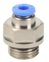
NITRA pneumatic push-to-connect fitting, male, straight, nickelplated brass body, nickel-plated brass threads, 5/32in (4mm) tube to G1/4 BSPP connection(s). Package of 5.
