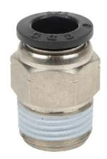
NITRA pneumatic push-to-connect fitting, male, straight, nickel-plated brass body, nickel-plated brass threads, 3/8in tube to 3/8in NPT connection(s). Package of 5.
