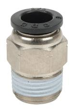
NITRA pneumatic push-to-connect fitting, straight, nickel-plated brass body, nickel-plated brass threads, thread sealant, (1) 3/8in male NPT to (1) 3/8in push-to-connect. Package of 5.
