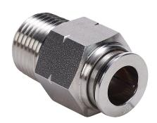
NITRA pneumatic push-to-connect fitting, male, straight, 316 stainless steel body, 316 stainless steel threads, 3/8in tube to 3/8in NPT connection(s).
